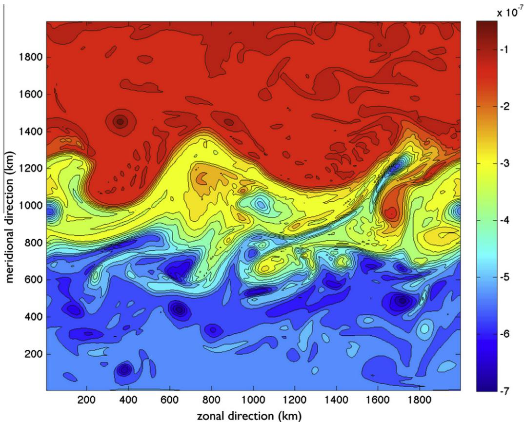
**Fig. 1.** A snapshot of PV in the upper ocean layer at day 6000 from the reference simulation. Strong PV gradients exist along the core of the meandering jet. PV filaments are shed, resulting in occluded PV cores that, on average, slowly propagate to the west.
