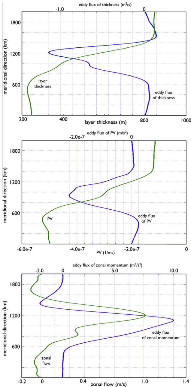
**Fig. 2.** All panels show eddy flux and mean state for the upper ocean layer. Panel A: The eddy-induced meridional flux of thickness,  $\overline{v'h}$ , along with the zonal-mean, time-mean thickness field. Panel B: The eddy-induced meridional flux of potential vorticity,  $\overline{(hv)'q}$ , along with the zonal-mean, time-mean potential vorticity field. Panel C: The eddy-induced meridional flux of momentum,  $\overline{(hv)'u}$ , along with the zonal-mean, time-mean zonal wind field.
