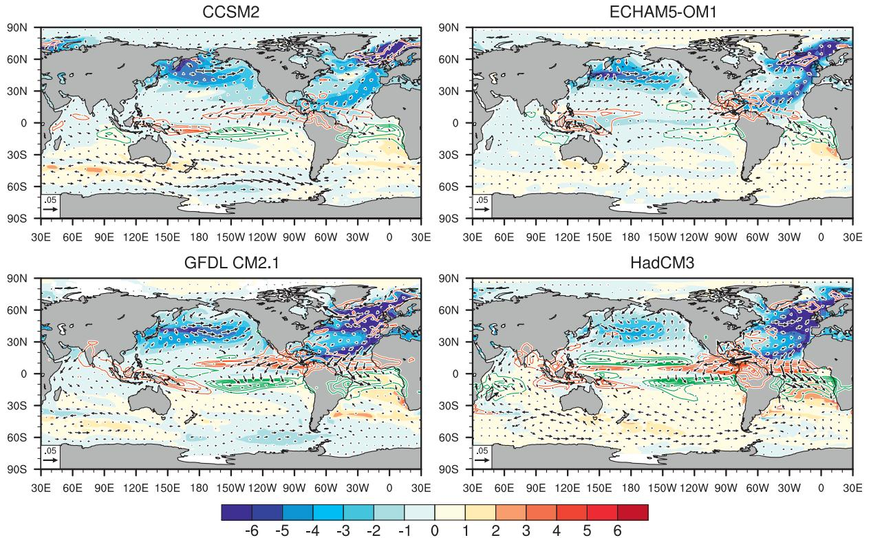
FIG. 1. Ocean–atmosphere anomalies simulated by four different coupled GCMs in the 1-Sv water-hosing experiment: SST (shading, °C), surface wind stress (vectors,  $\text{N m}^{-2}$ ), and precipitation (green contours  $> 1 \text{ mm day}^{-1}$  and orange contours  $< -1 \text{ mm day}^{-1}$  at intervals of  $1 \text{ mm day}^{-1}$ ) anomalies are averaged over the last 30 yr of the 100-yr hosing period.
